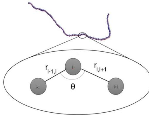
$$U_{\text{bond}} + U_{\text{bending}} + U_{\text{excludedvolume}} = \frac{\kappa_{\text{bonding}}}{2} \sum_{i=1}^{N_c} \sum_{j=1}^{N_i-1} (r_{j,j+1}^i - r_0)^2 + \frac{\kappa_{\text{bending}}}{2} \sum_{i=1}^{N_c} \sum_{j=1}^{N_i-2} (\theta_{j,j+1}^i - \theta_0)^2 + \sum_{\substack{\langle i,j \rangle \\ i < j, r_{ij} < \sigma_{ch}}} 4 \epsilon_{ch} \left\{ \left( \frac{\sigma_{ch}}{r_{ij}} \right)^{12} - \left( \frac{\sigma_{ch}}{r_{ij}} \right)^6 \right\}$$
